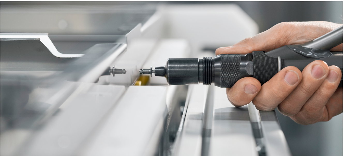
The blind riveting machines from GESIPA® are specially designed for use in industrial production, wherever many rivets have to be set efficiently in a short time.
